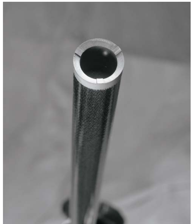
Figure 4: CFC-tube with carbide 3-point contact
